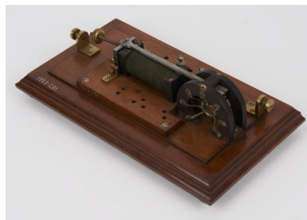
Ratchet switch fitted in theatres and used to switch the power to the microphones (Copyright London Science Museum)
