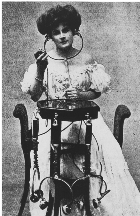
Electrophone user using a Transmitter No. 17 to talk to the Electrophone operator
