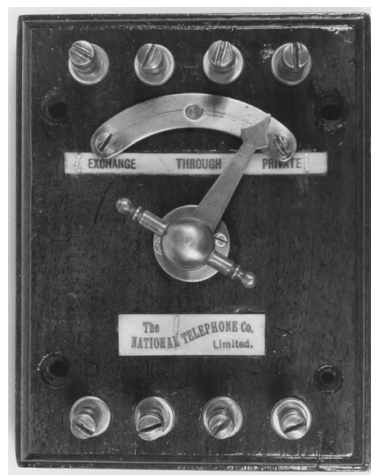
NTC Intermediate switch (Telephone to Electrophone switch)
