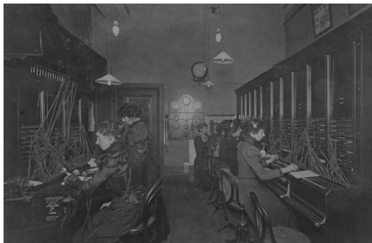
Early exchange in use - note the cords above the switchboard
