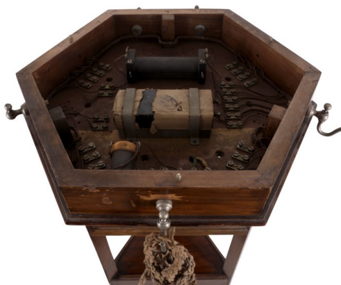
Electrophone table with top removed
